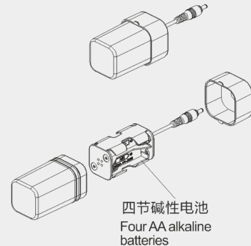
Step 1: Remove the battery box and remove the battery box cover.
