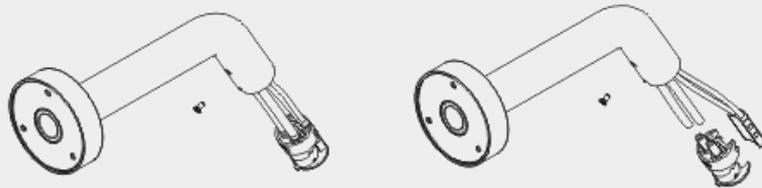
Step 1: Use the "hexagonal" wrench to take out the screw fixing the soap bubbler. Disconnect the hoses and the bubbler, and take out the soap bubbler.
